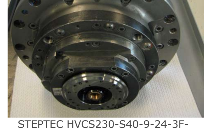
STEPTEC HVCS230-S40-9-24-3F-HSKA63-F80 24.000rpm
