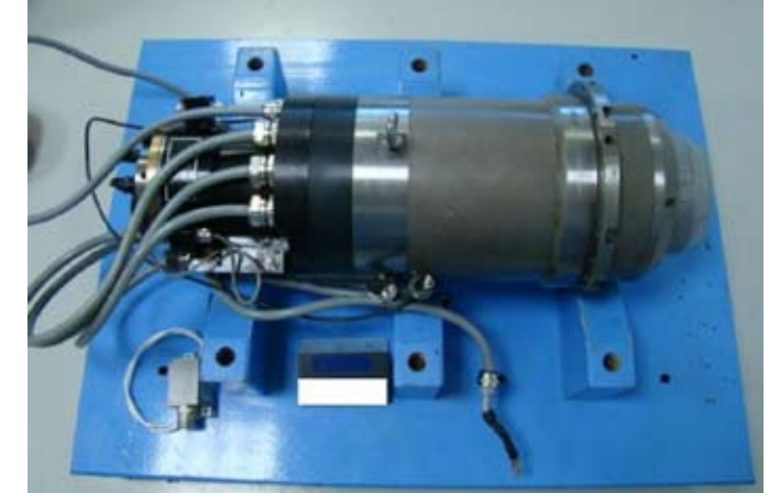
KESSLER DMS100 AL4 FOS SK40 12.000rpm
